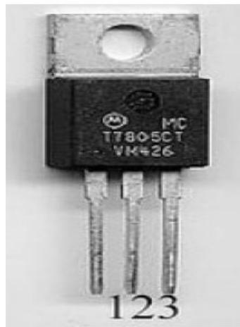
Pinout of the 7805 regulator IC
